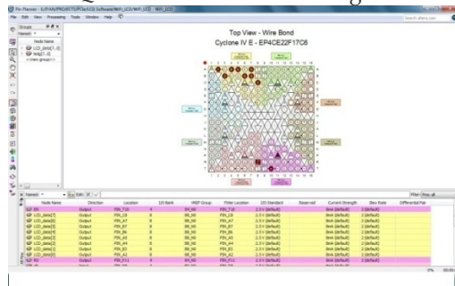
Fig 10 – Descriptive View of pin Assignment in Quartus .
